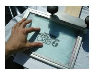
With the right equipment printing 'off contact' is no harder than direct (fabric) printing. The best thing you can do is to make the process fast and easy is to invest in a screen printing jig which will provide the correct height adjustment and accurate registration of the print.
