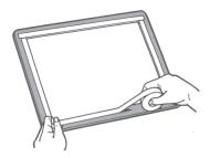
RISO ScreenMaster and EZIscreen StencilPro films use the same mounting process for each mesh type. Neither mesh is stretched onto the frame as with traditional silk screen mesh - it already has the emulsion attached and therefore is already pre-tensioned and does not require mechanical stretching to a frame. Over stretching the mesh will distort the design and reduce print quality.
